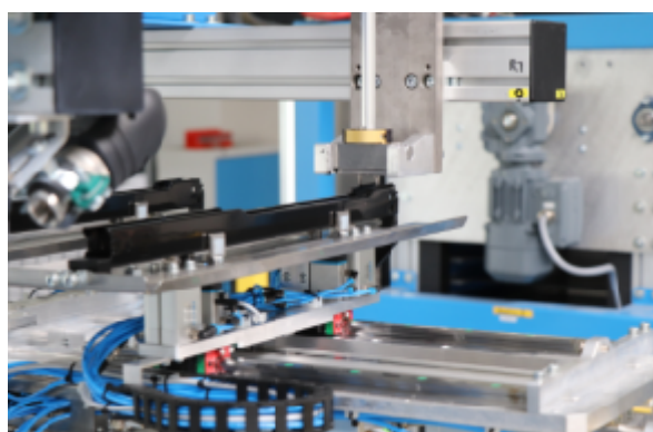
Automated bonding process in the production of oven doors
