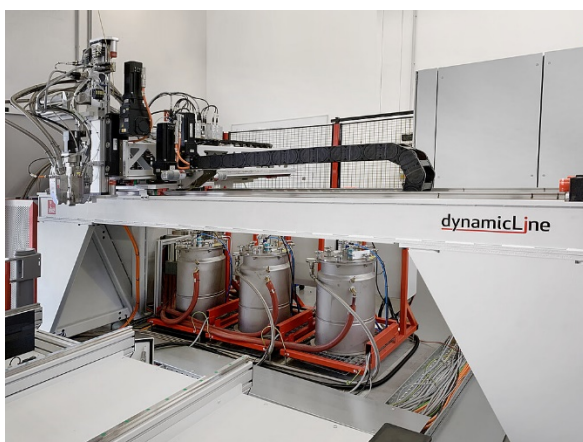
dynamicLine system for automated bonding and gasketing of control cabinets (doors, window panes, ventilation grilles); two shuttle sliding tables ensure efficient production
