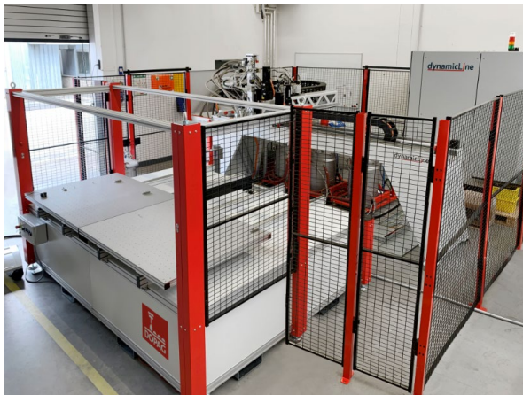
dynamicLine system for automated bonding and gasketing of control cabinets (doors, window panes, ventilation grilles); two shuttle sliding tables ensure efficient production
