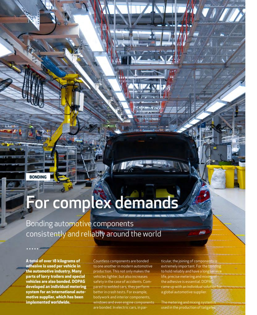
This involves bonding a plastic component to a metal or composites panel. The eldomix metering and mixing system from DOPAG is used, which is ideal for bonding applications and can be easily integrated into the highly automated production lines in the automotive industry. A dual-component polyurethane is metered and mixed. In the application, a robot with a speed of 300 cc/min places a bead around the trim of the tailgate with maximum precision.
