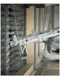
Everything is fully automated in the production hall: the photovoltaic modules are bonded to the metal frame with the eldomix metering and mixing system. The material is supplied via gear pumps. They are then assembled into a complete retractable roof group.
