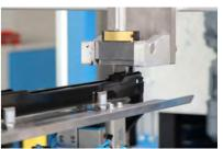
Above: Automated application of adhesive to components for the production of oven doors. Pre-treatment with Pyrosil has already been carried out
