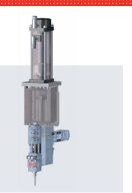
The vectodis metering system is suitable for processing single-component media. The material is discharged in shot or bead form. The material is taken from the original container via a feed pump and fed to a piston metering unit with a servo motor. A material pressure regulator keeps the input pressure at the piston metering unit constant.
