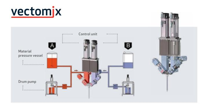
The vectomix is used to handle multi component materials. Due to its compatibility and modularity, two vectodis single component piston metering systems with equal or different sizes are used. They can be connected by simply using a mixing block onto the outlet of which a disposable plastic mixer is mounted. The use of a hose package with a decentralized mixing system is also possible. Just a suitable material supply and metering computer is required.
